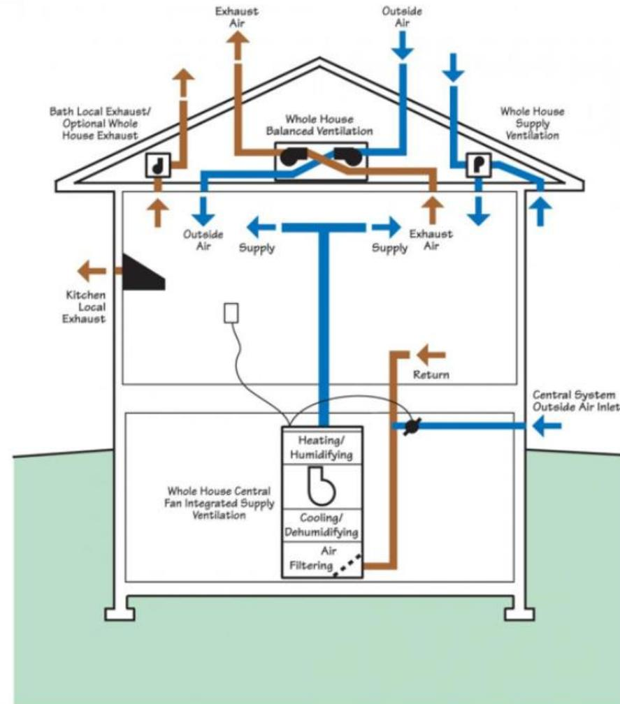
Figure 1. Examples of whole-house and local ventilation systems.
