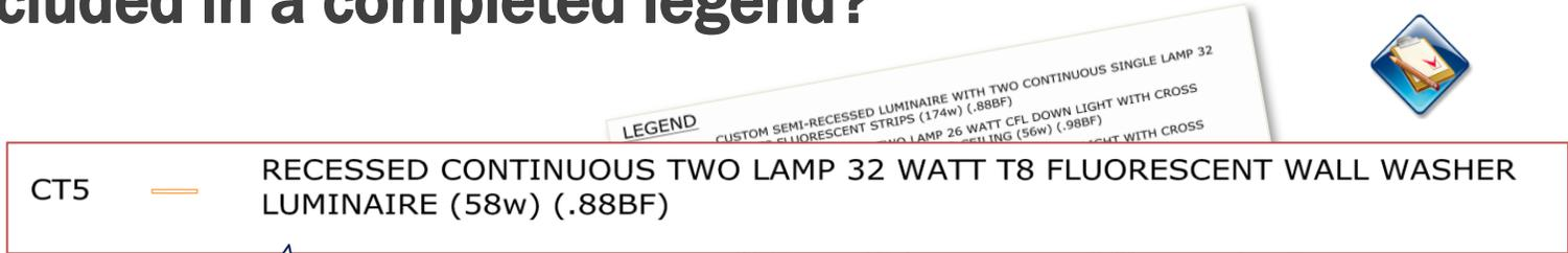
Specific information must be included. Ballast/transformer/driver types must be known to understand system watts (this is often missing in Legends).
