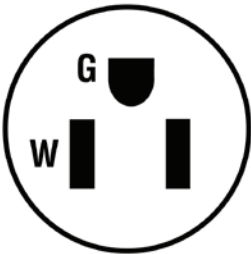
NEMA5 115V receptacle used on 115V units.
