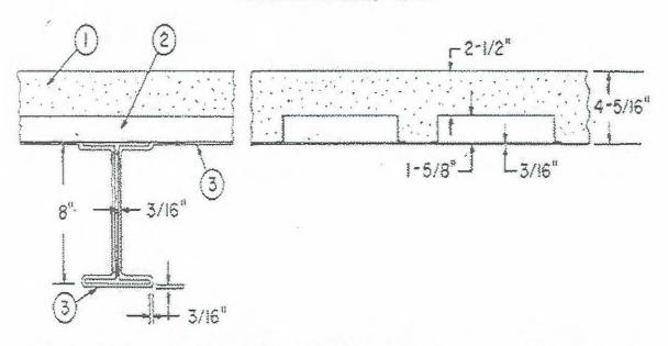
Steel Beam — Min size W8x17, with outside dimensions of 8x5 1/4 in, with a flange thickness of 5/16 in., a web thickness of 1/4 in., and a cross-sectional area of 5.01 sq in.
