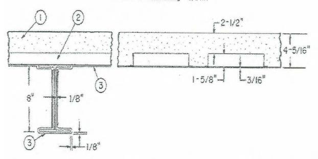
Steel Beam — Min size W8x17, with outside dimensions of 8x5 1/4 in. with a flange thickness of 5/16 in., a web thickness of 1/4 in., and a cross-sectional area of 5.01 sq in.
