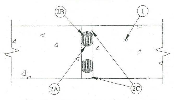
1. Wall Assembly — Min 4-1/2 in. thick reinforced lightweight or normal weight (100-150 pcf) structural concrete. Wall may also be constructed of any UL Classified Concrete Blocks\*.
