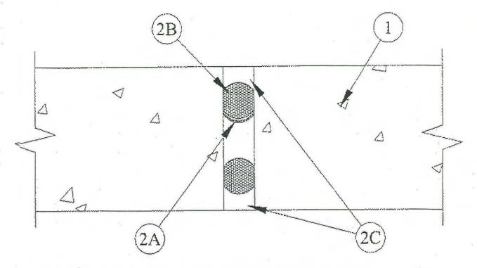
1. Wall Assembly — Min 4-1/2 in. thick reinforced lightweight or normal weight (100-150 pcf) structural concrete. Wall may also be constructed of any UL Classified Concrete Blocks\*.
