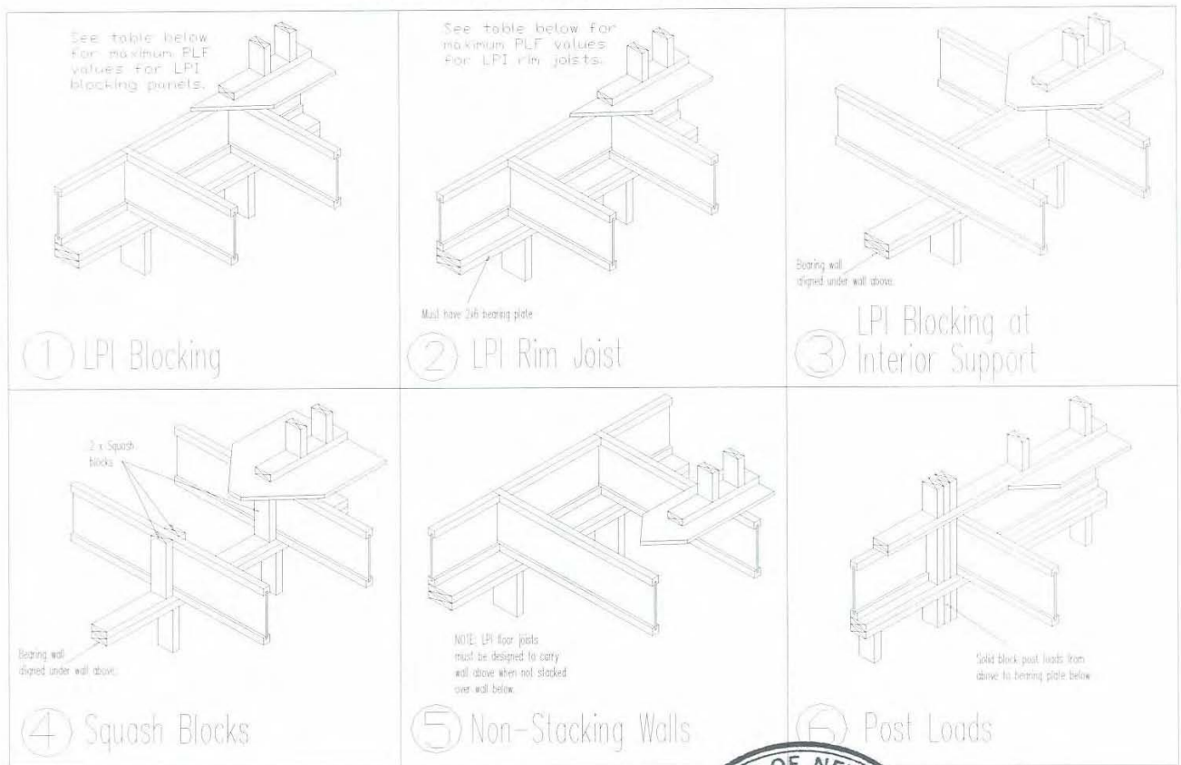
FIGURE 4 – I-JOIST FLOOR FRAMING DETAILS
