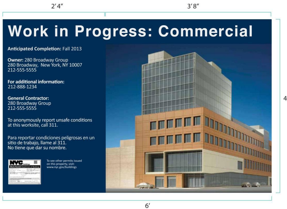
12 13 FIGURE 3301.9.1.4(2) 14 FENCE PROJECT INFORMATION PANEL LAYOUT 15 For SI: 1 inch = 25.4 mm, 1 foot = 304.8 mm.
