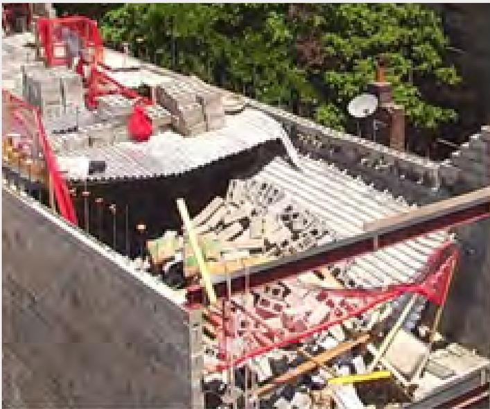
CMU blocks were stacked on a deck supported by cold-formed joists without adequate shoring, overloading the deck.
