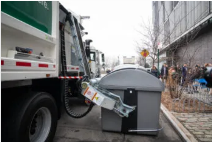
The new sanitation trucks will be able to lift these larger containers which help remove the piles of trash bags off city streets. Image Credit: Ed Reed/Mayoral Photography Office.
