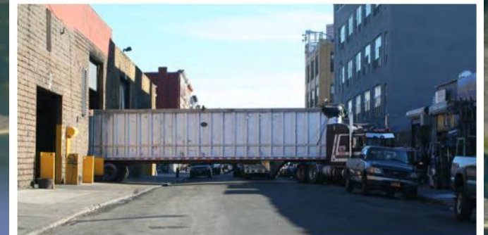
Difficulty backing trucks into loading berths on narrow streets
