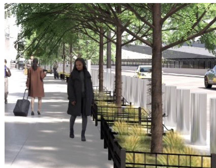
Curbside rain gardens, street trees, and bollards
