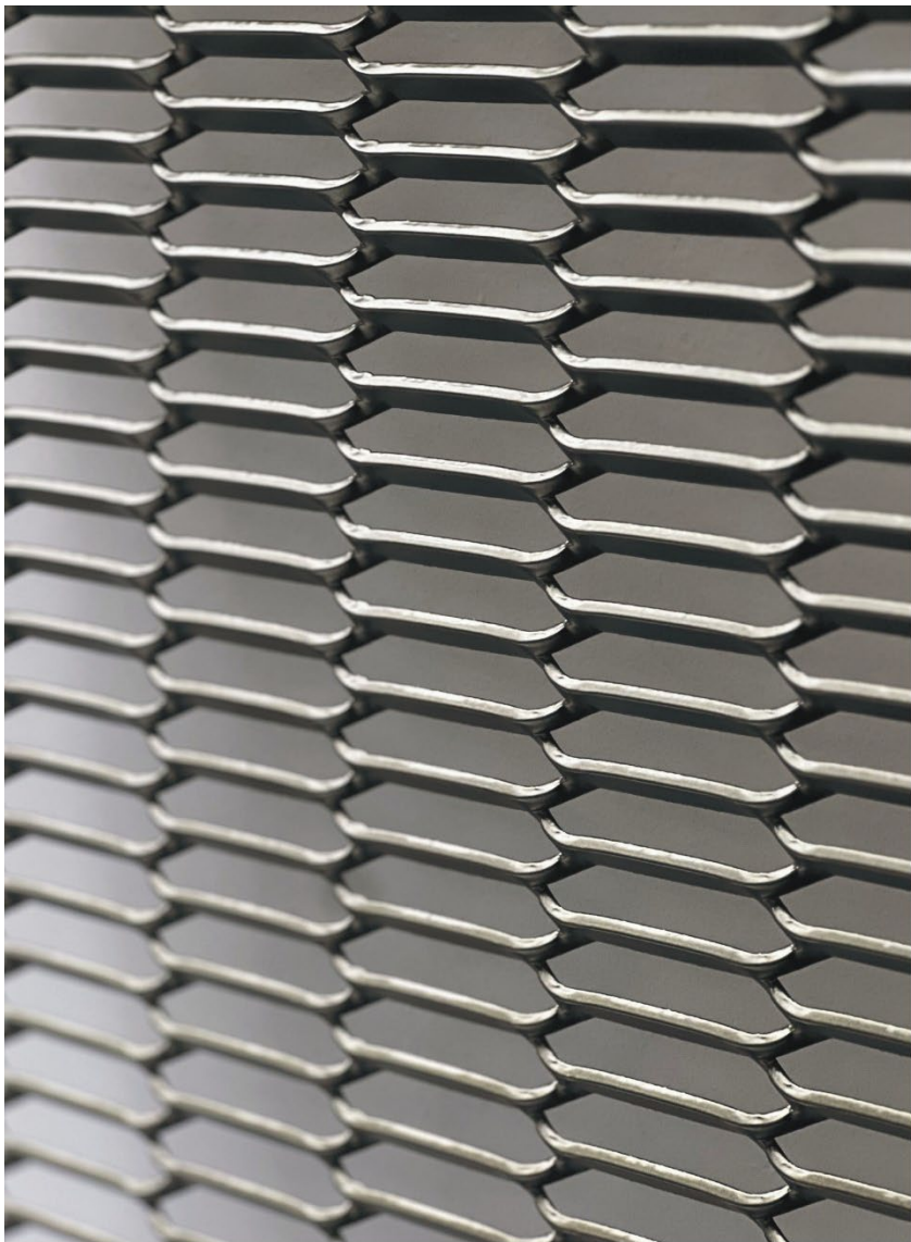
OBLIQUE VIEW OF EXPANDED METAL ONLY
