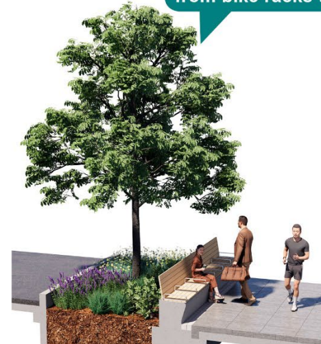
Crash Rated Concrete Seatwall with Planter
