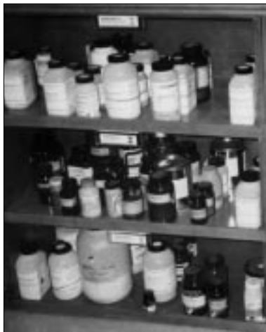
Low shelves with shelf labels, and proper labeling of all chemicals reduces accidents in chemistry labs.
