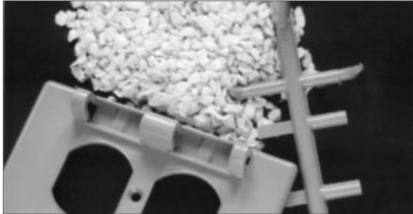
Runners (right) that hold the product (switch plate above) in the manufacturing process are reground and fed back into the process at a ratio of 25% regrind (top) to 75% virgin plastic resin.
