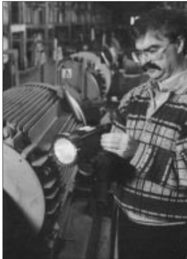
Measuring the speed of a motor can determine its efficiency and load. DOE's Motor Challenge Program can help.
