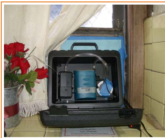
Sampling case with sampling pump (L), Sidepak (C) and PMI (R) installed in window.
