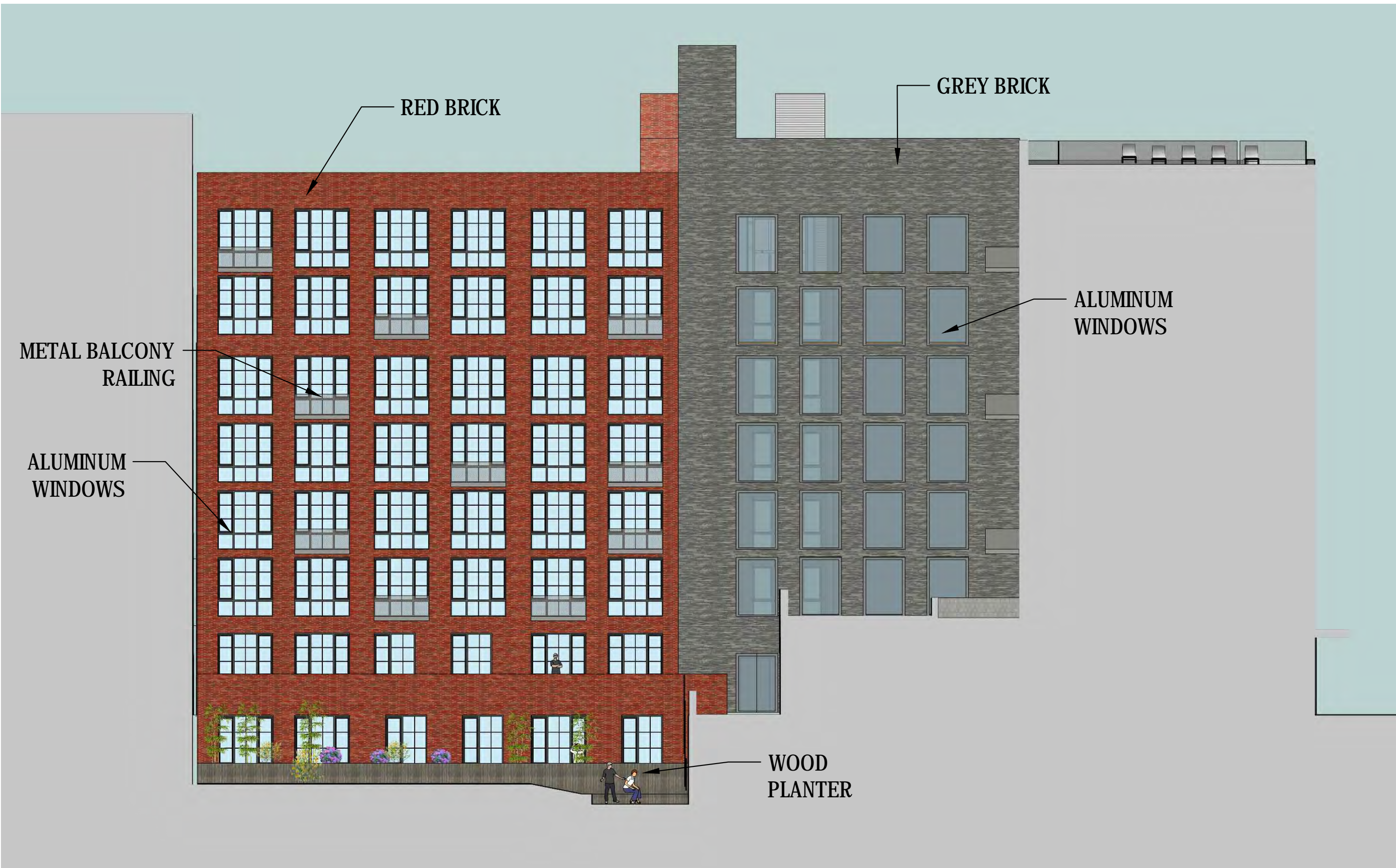
6 12TH STREET. COURTYARD ELEVATION SCALE: 1/8" = 1'-0"
