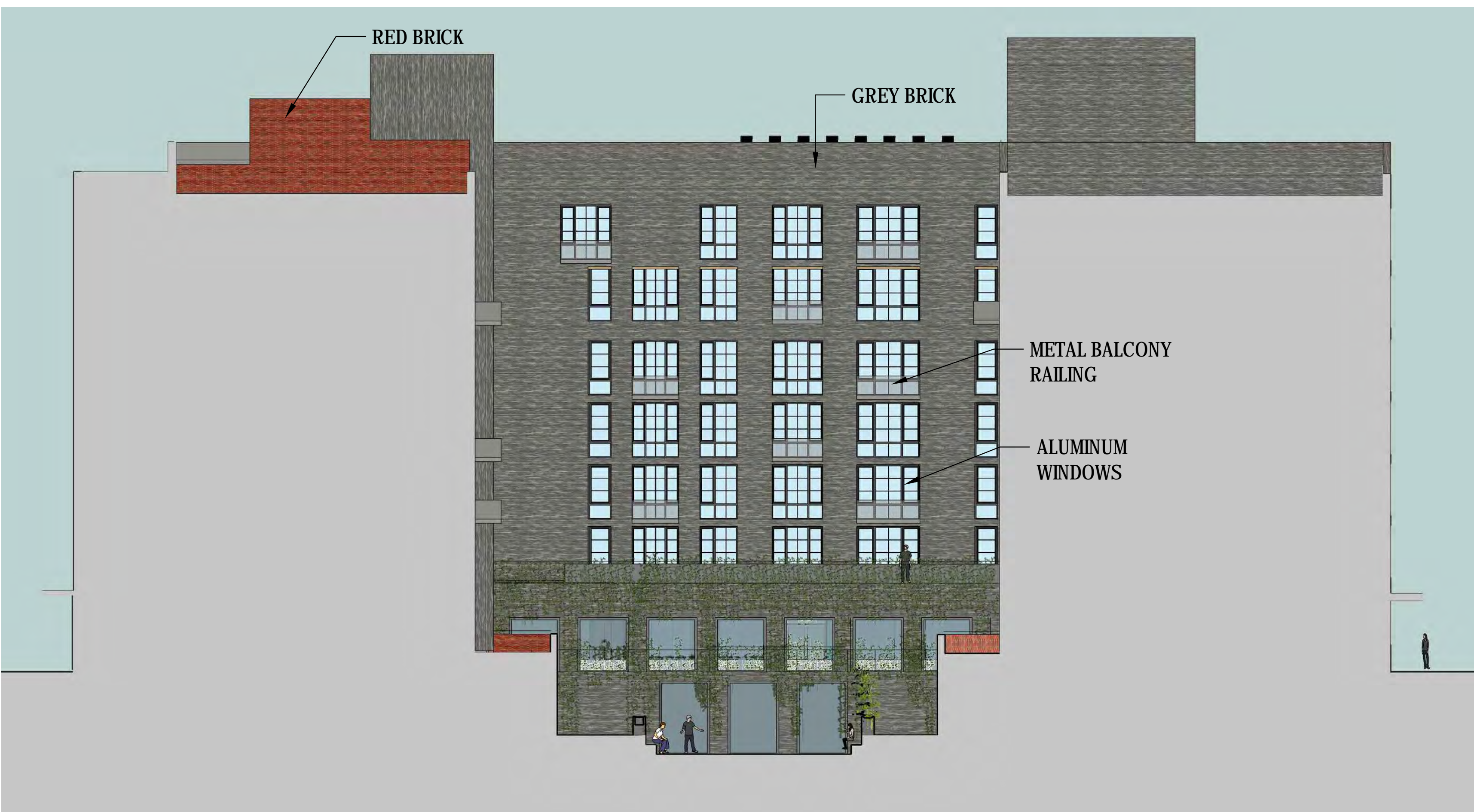
4 AVENUE A. COURTYARD ELEVATION SCALE: 1/8" = 1'-0"
