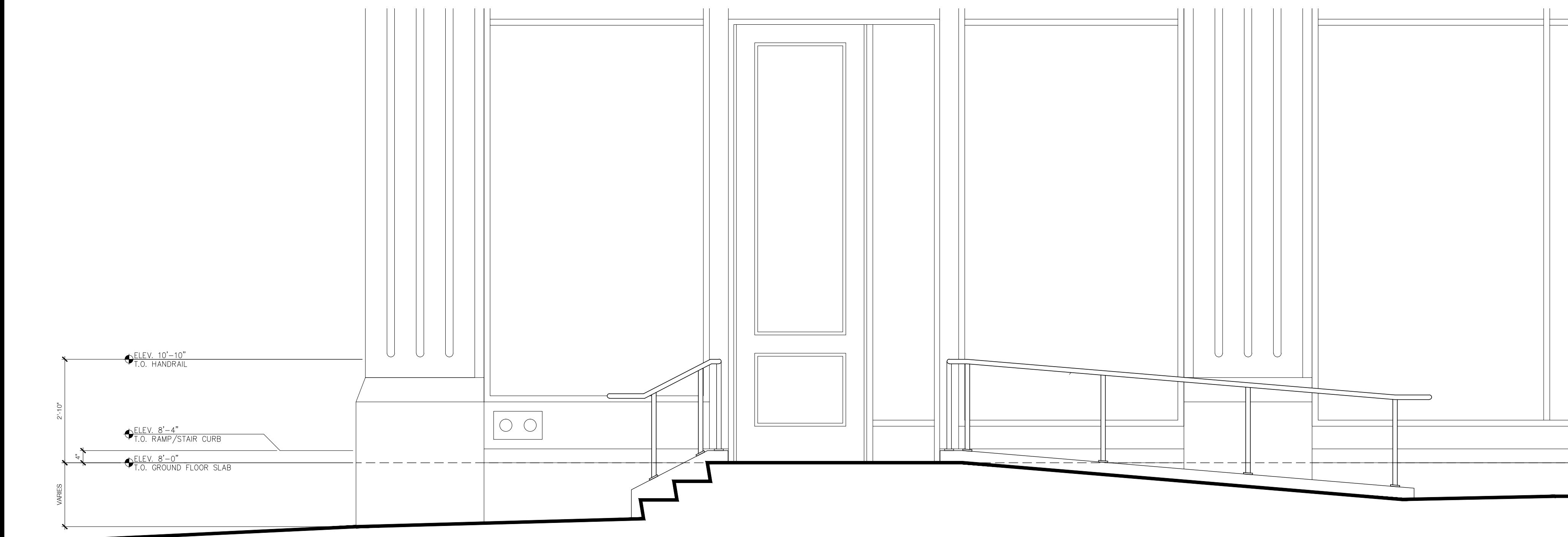
1 PROPOSED RAMP @ WEST BROADWAY ENTRY: PART SECTION ELEVATION SCALE: 3/4" = 1'-0"
