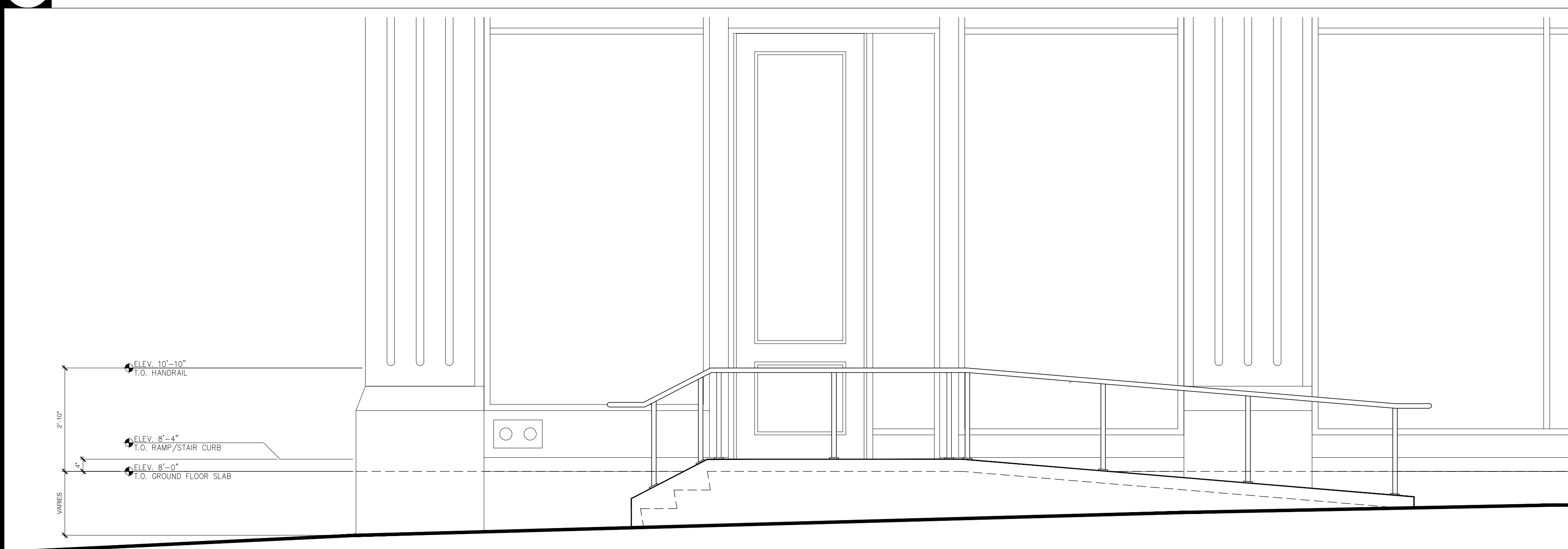
2 PROPOSED RAMP @ WEST BROADWAY ENTRY: PART ELEVATION SCALE: 3/4" = 1'-0"
