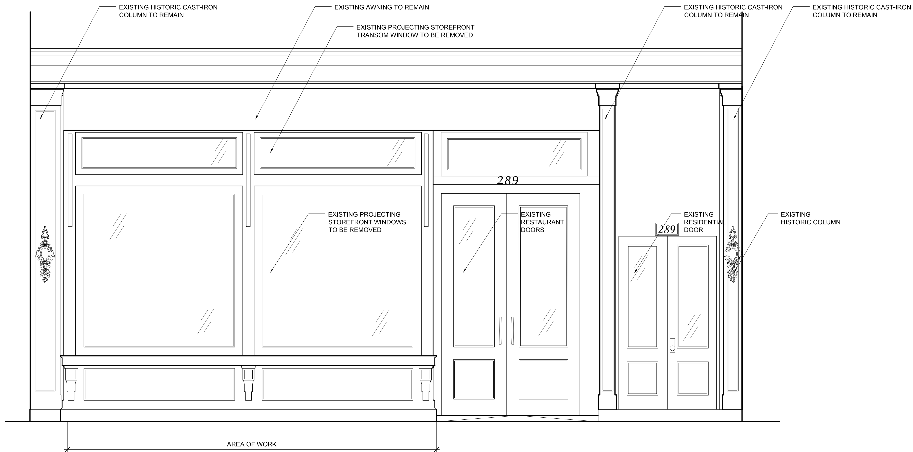
1 EXISTING FIRST FLOOR ELVATION SCALE: 1/2"=1'-0"
