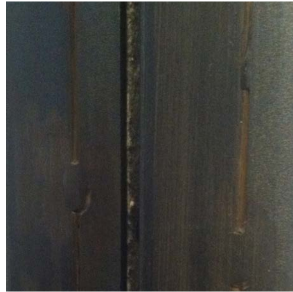
CLEAR-COATED IRON: PAINTED STEEL FOR ALL DOOR + WINDOW FRAMING, ENTRY DOOR HARDWARE + EXTERIOR LIGHTING
