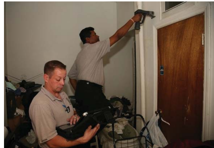
Housing Inspectors use an x-ray fluorescence analyzer to detect lead in the paint on a wall.
