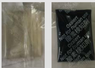
Oxalert™ integrity indicator is clear product is okay to use Oxalert™ integrity indicator is black discard product
