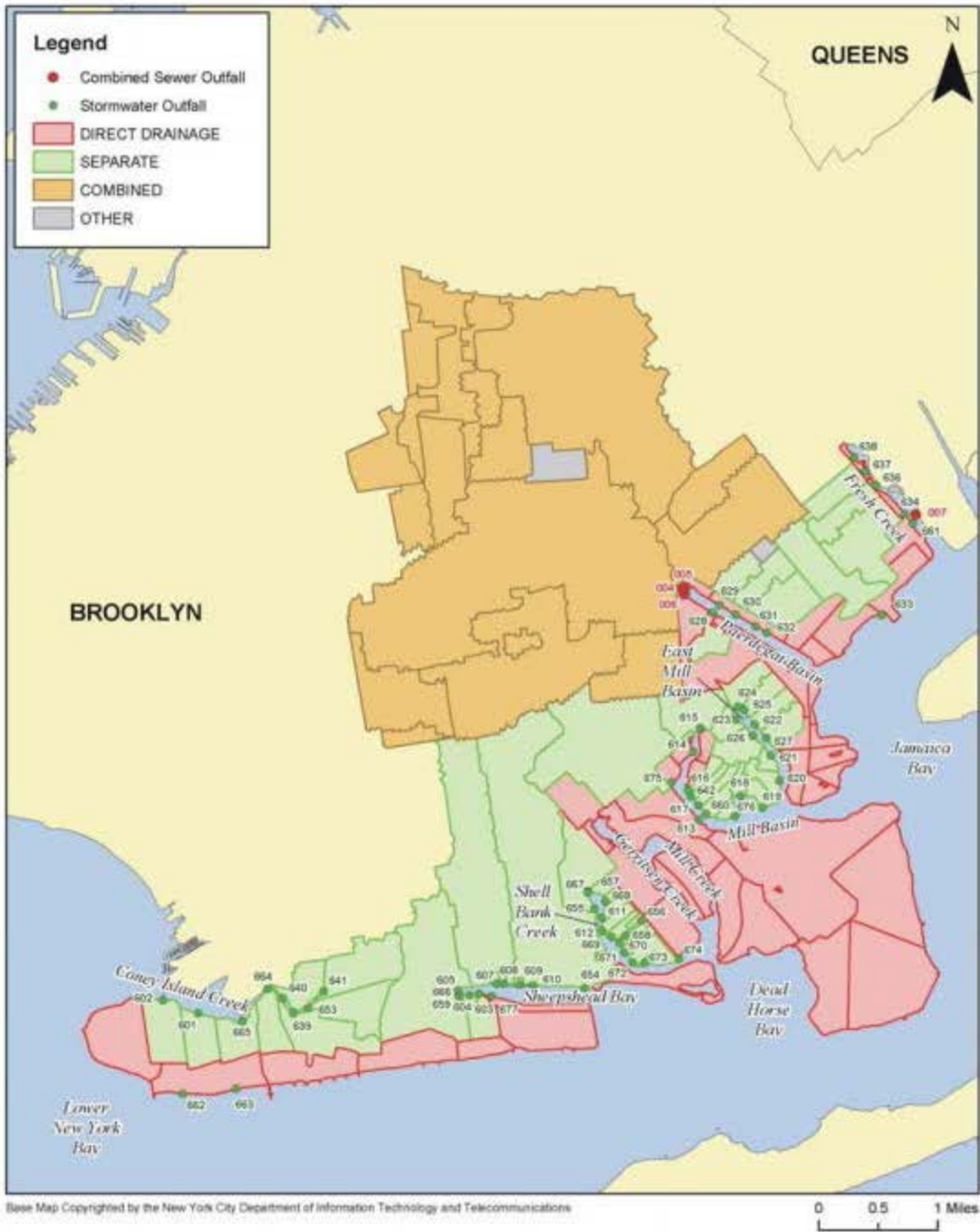
FIGURE 3. SCHEMATIC OVERVIEW OF THE CONEY ISLAND WPCP DRAINAGE NETWORK, CONEY ISLAND HOSPITAL IS IN THE DRAINAGE AREA TO 641 OUTFALL AT CONEY ISLAND CREEK, NYCDEP LANDSIDE MODELING REPORT, OCTOBER 2007.
