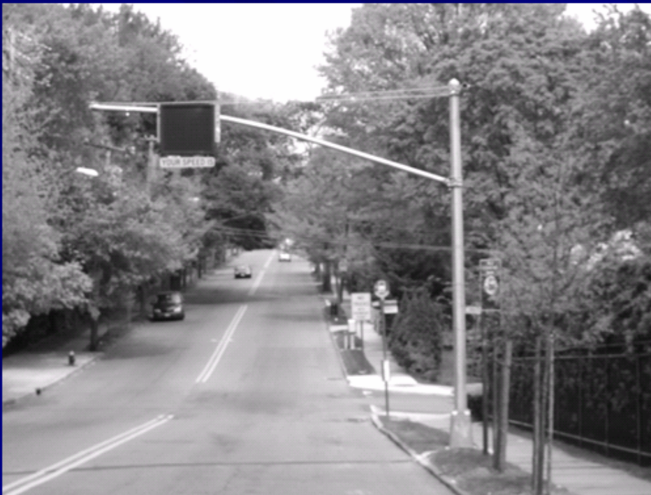
Photo illustrating Speed Boards on Henderson Avenue Corridor to improve safety and reduce vehicular speeding, 6/15/06 NYCDOT.
