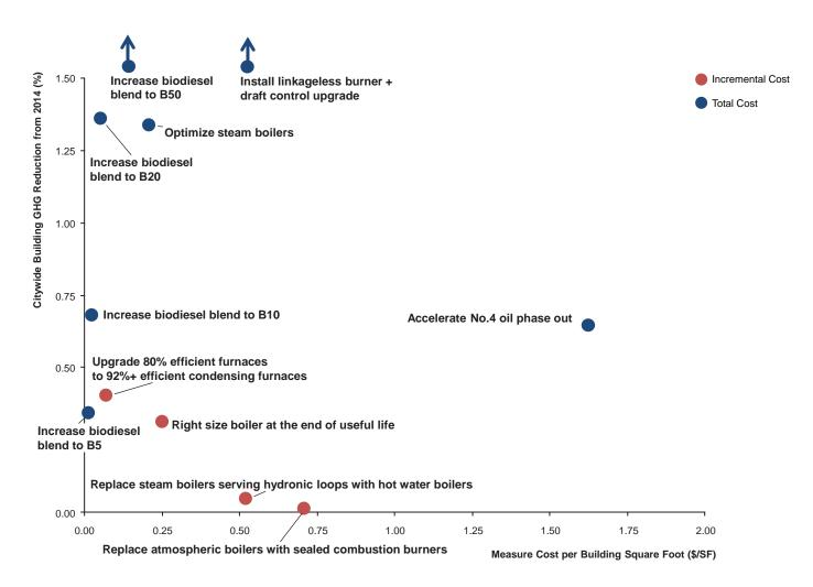
Heating equipment includes the boiler, furnace, or other mechanical means to generate space heating for a building. This category does not include the heating distribution system, which distributes space heating throughout a building, or the DHW system, which produces hot water. Because the energy used for space heating is the most significant end use in New York City buildings and heating equipment is found in every building, many of these ECMs could yield significant citywide GHG reductions.
