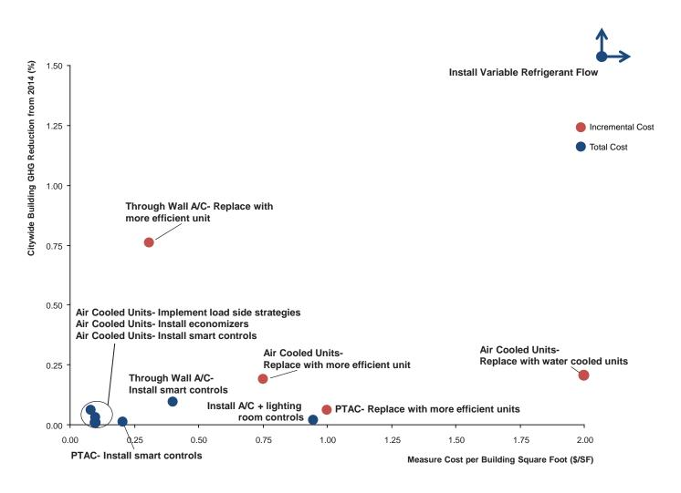
Non-central cooling systems provide cooling to individual rooms or specific zones of a building. These systems include PTACs, window air conditioners, through-wall air conditioners, and air-cooled packaged units (ACPUs). Non-central cooling systems are much more common than central cooling systems in New York City buildings, particularly in residential buildings and in pre-war commercial buildings.
