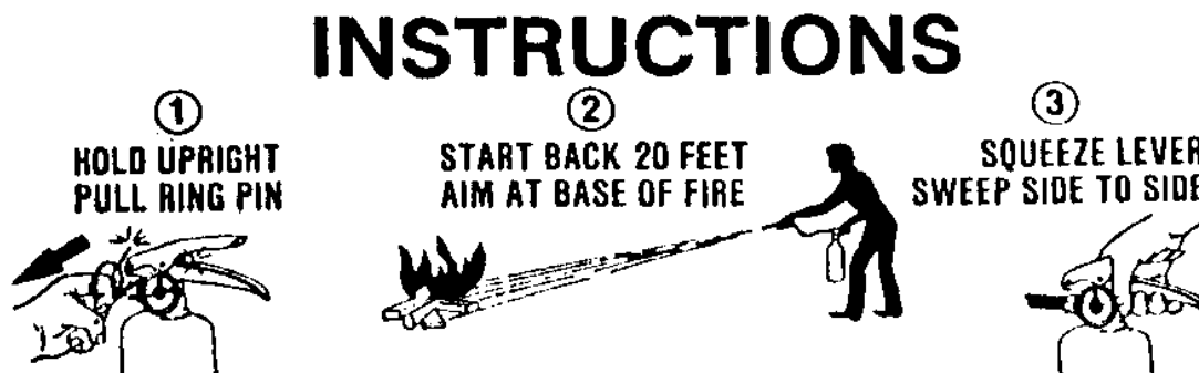
Typical Instructions for Using the Fire Extinguisher
