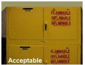
provided with a conspicuous label in red letters on contrasting background which reads: FLAMMABLE-KEEP FIRE AWAY. The door must be well fitted, self-closing and equipped with a three-point latch. The bottom of the cabinet must be liquid-tight to a height of at least 2 inches.
