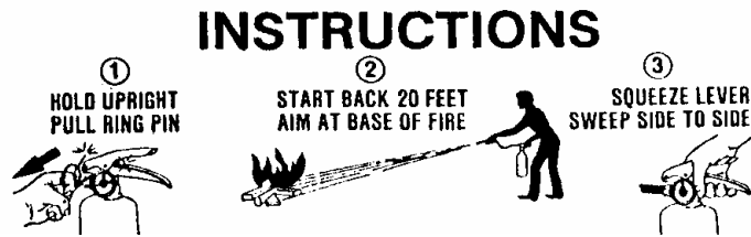
Operation Instructions for a Fire Extinguisher
