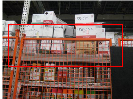
Improper stacking of combustible cartons above aerosol storage area
