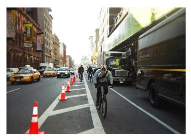
traffic cones were used citywide to separate bicycle and vehicular traffic and a Standing" "No regulation was placed on each of the abutting curbsides. Between the hours of 5am and 8pm, two shifts of personnel monitored the cones. However, there was a high incident of illegal parking and noncompliance on the extended bike lanes due to vehicles parking along the curb or vehicles using it as a through lane. The bicycle network in the other boroughs was also promoted (also included in Appendix
