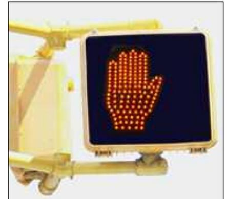
**Traffic Signal/Pedestrian Signal:** The red, yellow and green lights, as well as the pedestrian signals (with the symbolic **Walking Figure=WALK** and **Raised Hand=DON'T WALK**), are designed to let people in vehicles and on foot know who has the right-of-way. Traffic signals help manage traffic flow on main and cross streets, and help pedestrians cross an intersection safely.
