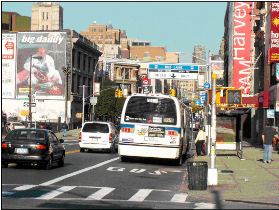
Dedicated bus lanes and newly designed overhead signs were installed to make bus lanes more prominent.
