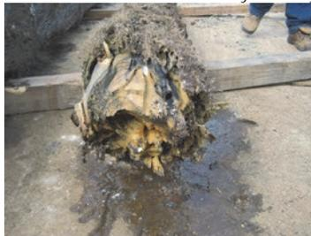
During the Demolition of the North End of the Existing University Heights Bridge Fender, Marine Borers were Discovered in the Southern Yellow Pine Piles. The End of a Pile Segment Removed From the Fender - Based on the Size of the Holes, *Teredo Navalis* is the Likely Species.
