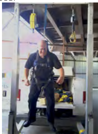
Associate Project Manager Thomas Whitehouse Hoisted in the Air While Wearing a Full Body Harness - Demonstrating How to Deploy and Use the Foot Stand to Prevent Orthostatic Intolerance (Commonly Referred to as Suspension Trauma), Which Can be Fatal if Not Prevented. (Credit: Gean Pilipiak)
