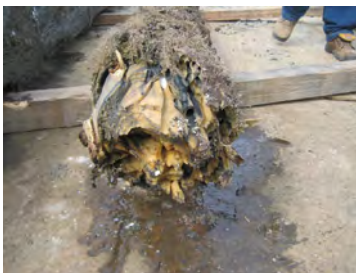
During the Demolition of the North End of the Existing University Heights Bridge Fender, Marine Borers were Discovered in the Southern Yellow Pine Piles. The End of a Pile Segment Removed From the Fender - Based on the Size of the Holes, Teredo Navalis is the Likely Species.
