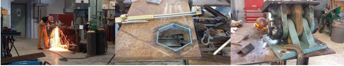
July 2014: Supervisor Bridge Repairer and Riveter Steve Havemann Fabricating a Wrench to Remove Nuts From a Seized Rocker Bearing.
