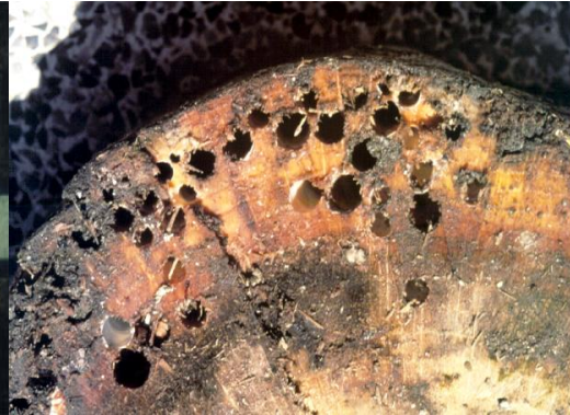
Teredo Damage (holes up to 1/4" diameter)
