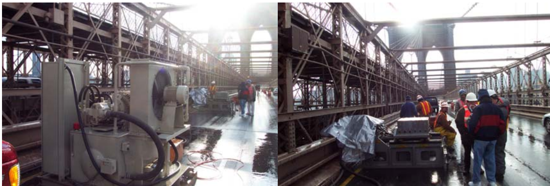
Measuring Ambient Vibrations on the Bridge. (Credit: Bojidar Yanev)
