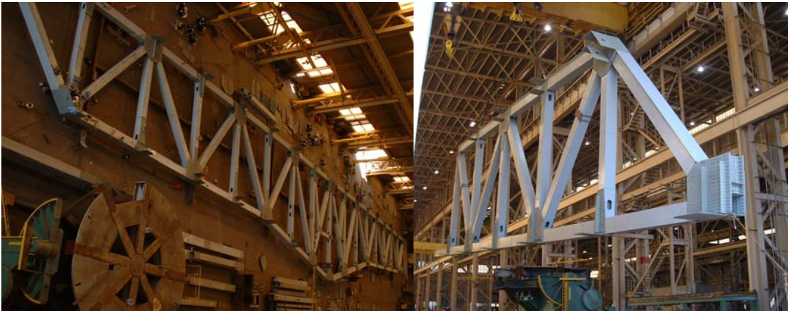
Third Avenue Bridge Truss Fabrication in Alabama
