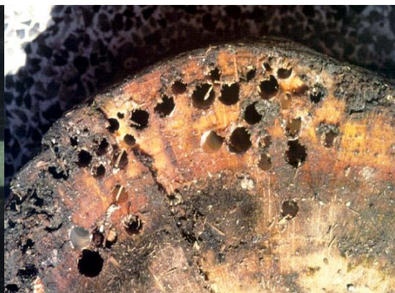
Teredo Damage (holes up to 1/4" diameter)
