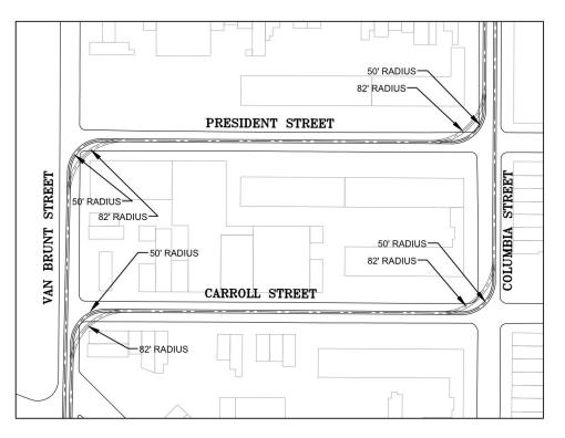
Figure 3-1: Horizontal Curvature (82 feet versus 50 feet)
