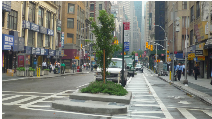
Example of pedestrian refuge island to be installed as safety improvement
