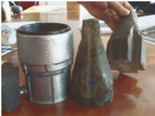
Under the NYC Electrical Code, metal, insulated collars (left) should be used to support electrical cables in high-rise buildings, not wooden chocks that Electrical inspectors found at five sites in Manhattan.
