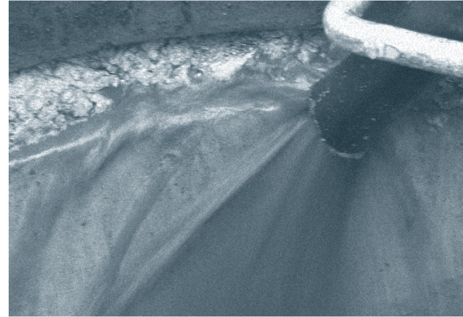
Biofilm and precipitated iron pumped from well
