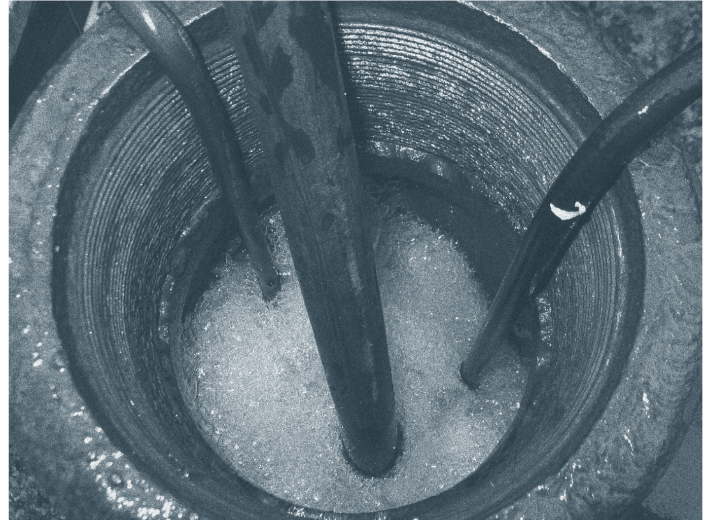
Impulse generation creating nitrogen bubbles at well head
