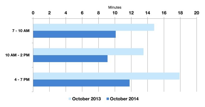
SBS trips are **32-34% faster** in bus lane section
