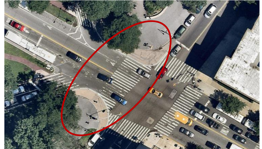
W 79 th St at Riverside Dr. curb extensions will be built out in concrete
