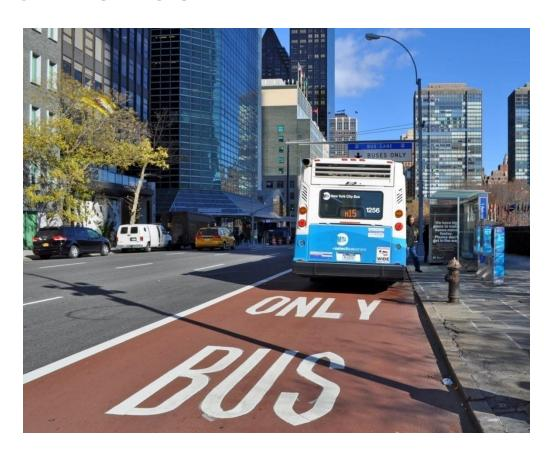
When the bus was in motion, bus lanes allowed SBS to move 11% faster than Limited
