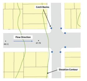
Figure 6.1. Example roadway flow direction analysis.
