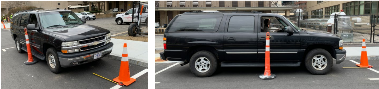
Figure 10. Setup for 3-foot and 4-foot cone method of blind zone measurement.
