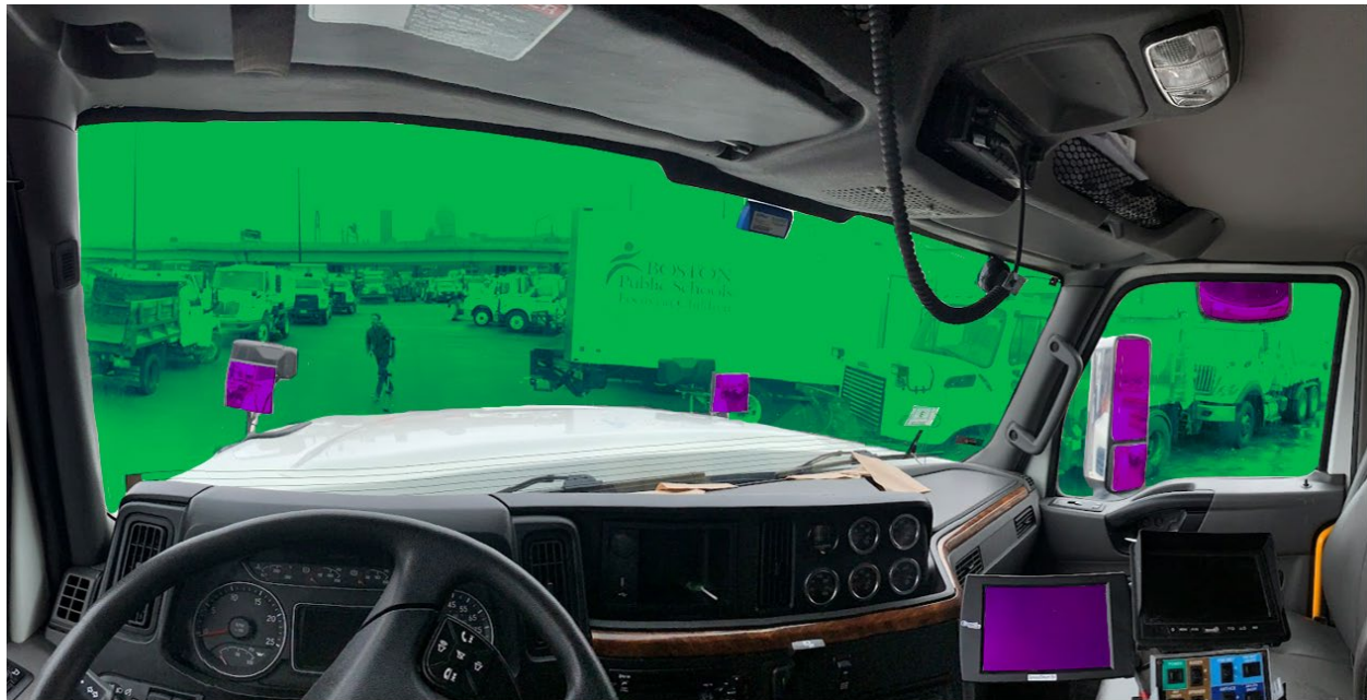
Figure 1: View from the driver's seat of an International HV 513. Direct vision of the environment is shaded green (unobstructed view through the windows) and indirect vision areas are shaded purple (mirrors and camera display unit).
