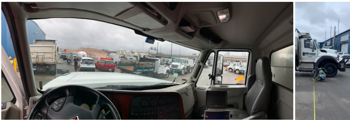
Figure 5. Left: Driver's view from measured International Workstar. Right: View toward driver from the nearest point at which the driver can see the road.
