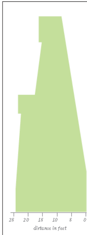
Figure 1 The above drawing represents a cross section of the Castle Village retaining wall after construction.
