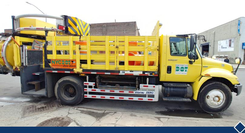
A side guard installed on a Department of Transportation truck.
