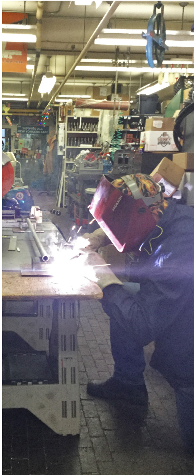
Joseph Jensen, from the DCAS plumbing shop, welds together light fixture parts.
