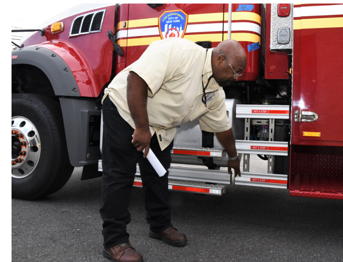
Fidelis Utulu, Deputy Director of Quality Assurance, ensures the Vision Zero side guards installed on the cable scrapper are the correct height to provide safety.
